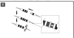
Insert the red and black wires into their housings. Secure the wires by turning the lock
